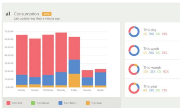
VRM Portal When the Inverter RS is connected to a GX device with internet connection, you can access our free remote monitoring website (VRM). This will display all your system data in a comprehensive graphical format. System settings can be changed remotely via the portal. Alarms can be received by email.
